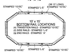
Place bottom rails stamped "L-S" between the side verticals. Place the bottom rails stamped "1015C" on the outside edge of the side supports as shown above. Place bottom rails stamped "A" on the ends of the pool.
