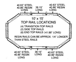
Refer to the diagram above for proper top rail placement. RESIN TOP RAILS CAN BE APPROX. 1/4" LONGER THAN STEEL TOP RAILS.
